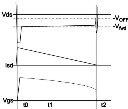
**Figure 4: Synchronous Rectification Operation at Light Load**
