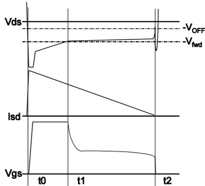
**Figure 3: Synchronous Rectification Operation at Heavy Load**
