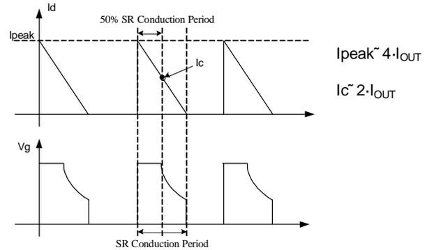
**Figure 6: Synchronous Rectification Typical Waveforms in QR Flyback**
