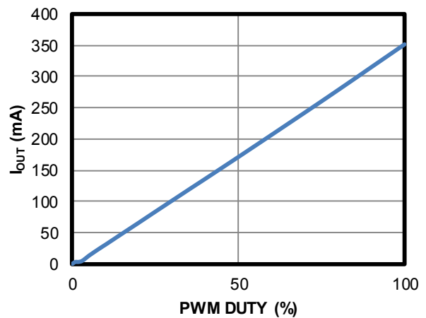
1kHz PWM Dimming Curve
