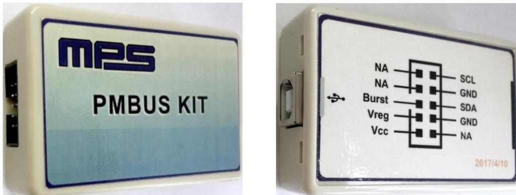
**Figure 3: EVHR1203 PMBUS Kit-01A Communication Interface**
