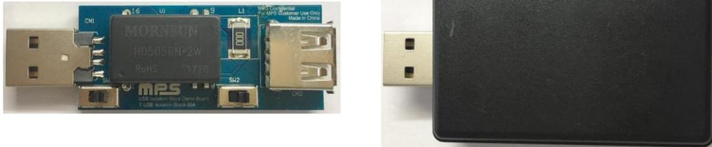
**Figure 4: T-USB Isolation Block-00A Isolator**
