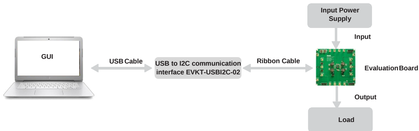
Figure 1: EVKT-5416 Evaluation Kit Set-Up
