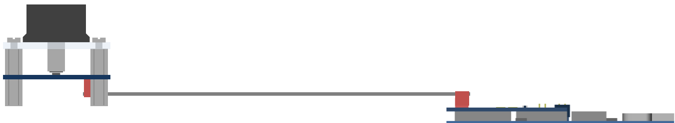
Figure 19: Connect EVKT-KNOB to EVMA-CONN board (view from the side)
