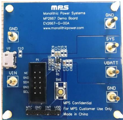
Figure 2: EV2667-G-00A Evaluation Board
