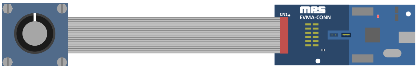
Figure 18: Connect EVKT-KNOB to EVMA-CONN board (view from the top)
